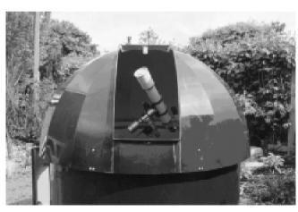
The main telescope is a Takahashi FS102, a 102 mm apochromatic fluorite refractor with a focal length of 820 mm. This is mounted on a Vixen Great Polaris DX. controlled by a Skysensor 2000 GOTO unit, and the whole lot is supported by a very solid pillar from BCF Astroengineering. The CCD camera is a Starlight Xpress MX716. The set up can be seen in Figure 1
