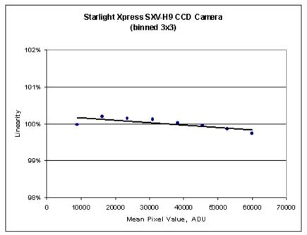
Figure 6, Linearity of SXV-H9 in 3x3 binned mode
